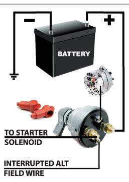
Designed to be installed right inline on your positive battery cable. Extra heavy-duty. Protects against theft and electrical failures. Install under your hood, seat on firewall or at the rear of the car. Rubber insulator boots cover stud and nut for the extra protection needed to prevent short circuits. Uses 3/4" mounting hole.
